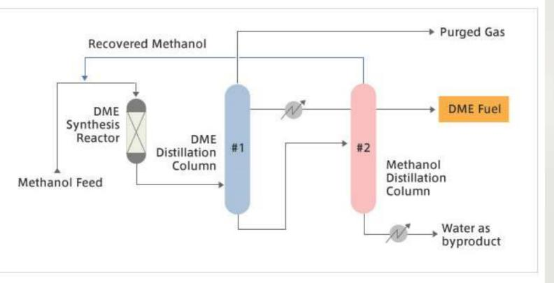
DME Synthesis Process (methanol dehydration)
